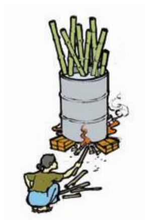
Heat treatment with preservatives
