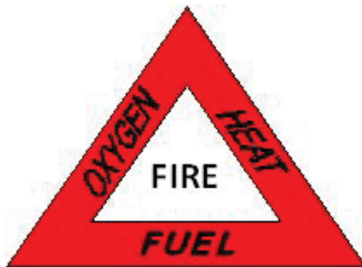
Figure 1.1: The three elements of fire
