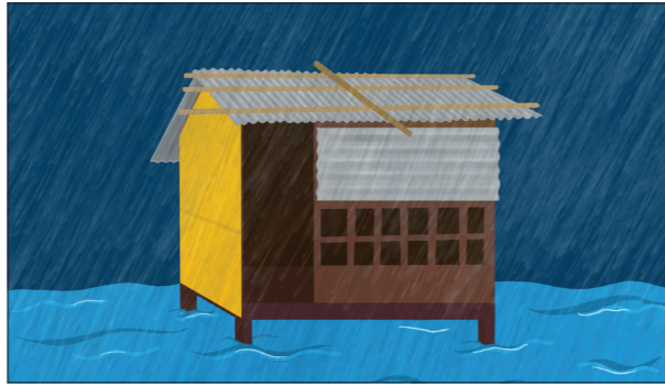
Photo showing the plinth level or foundation 2 to 3 feet above ground level.
